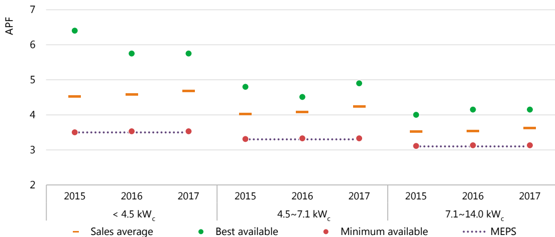
Figure 26. Range of energy performance for variable-speed mini-split ACs, 2015-17
