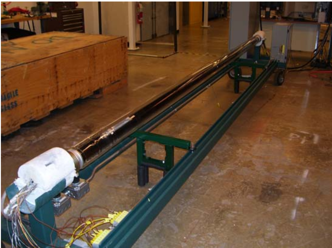
Figure 2. HCE heat-loss test stand at NREL
