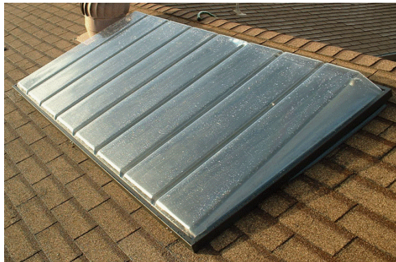
Fig. 2. DEG/SE glazed ICS on field test
