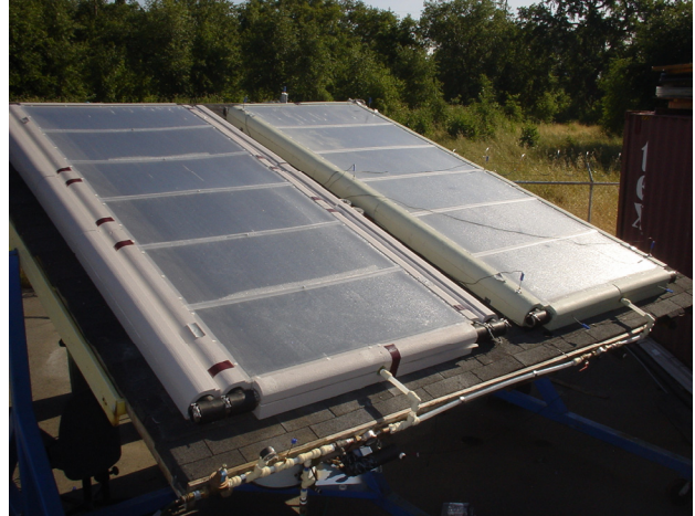
Fig. 4. Two thermosiphon prototypes on test at FAFCO
