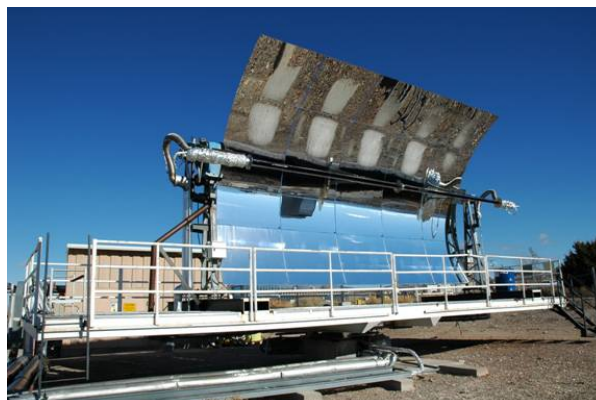
Fig. 2. Schott receiver on test at the NSTTF
