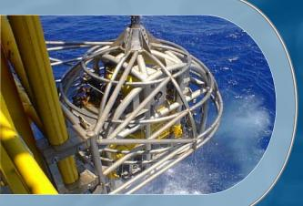
The side-entry cage, with a capacity of 600 ft of neutrally buoyant flying tether, provides protection during launch and recovery, makes deployment and recovery more efficient in marginal weather and high currents, provides additional tooling capabilities and storage, and provides additional payload for the deployment and recovery of subsea equipment.
