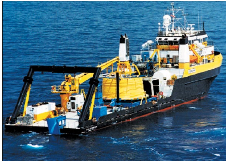
500 T carousel positioned for subsea tieback installation.
