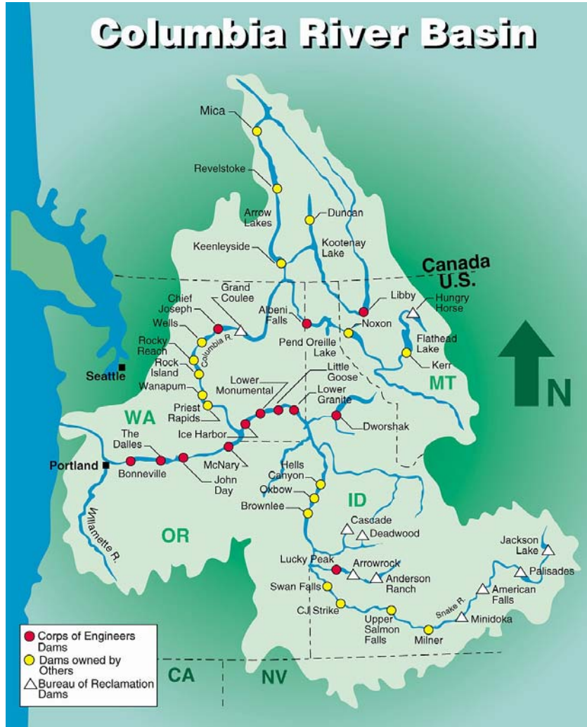
Figure 3.9. The hydropower dams of the Columbia River Basin are mostly run-of-river projects. (Map courtesy of U.S. Army Corps of Engineers.)
