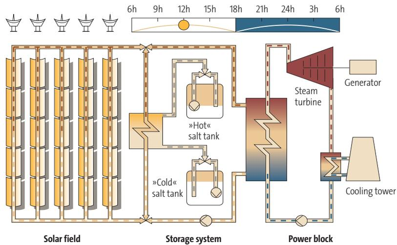
During the night, the power plant can be operated with the stored energy.
