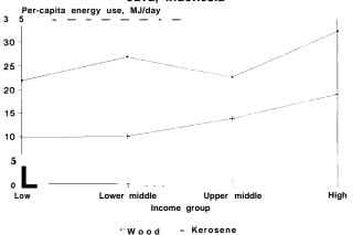
This figure compares energy use in households using only wood with that in households using only kerosene within the same income class. Households using kerosene consume roughly half as much energy as households using wood.
