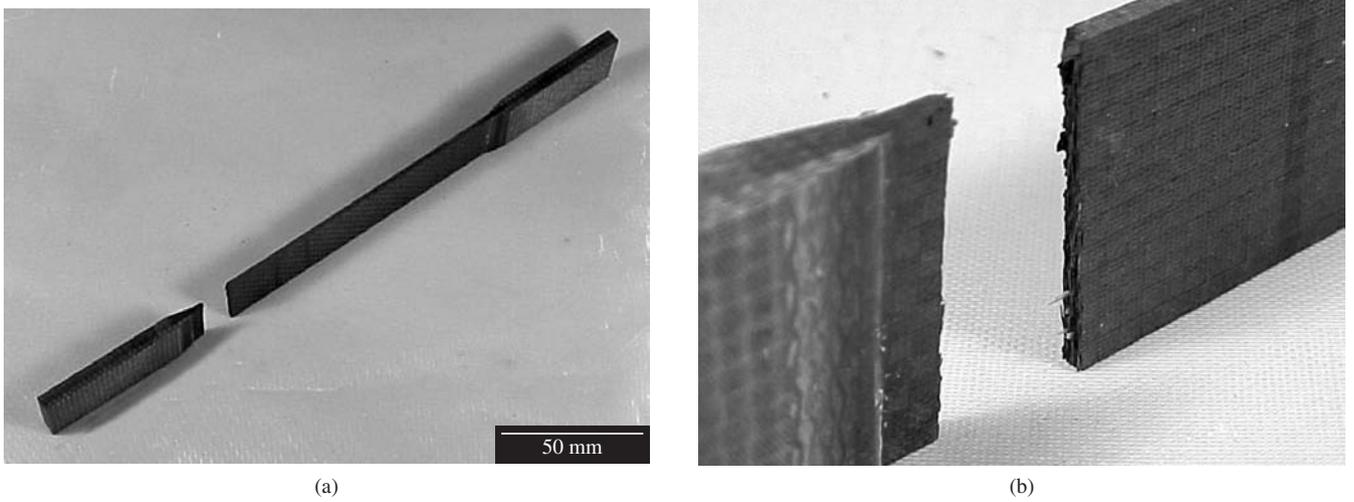
**Figure 6.** F584/PW laminate: a) specimen tested; and b) detail of the failure mode type LGB (**Lateral Gage Bottom**).
