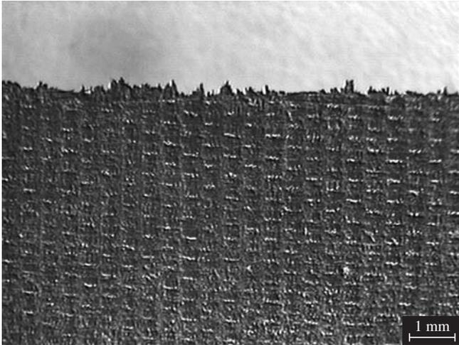
Figure 8. F155/PW specimen after tensile test, (10x).
