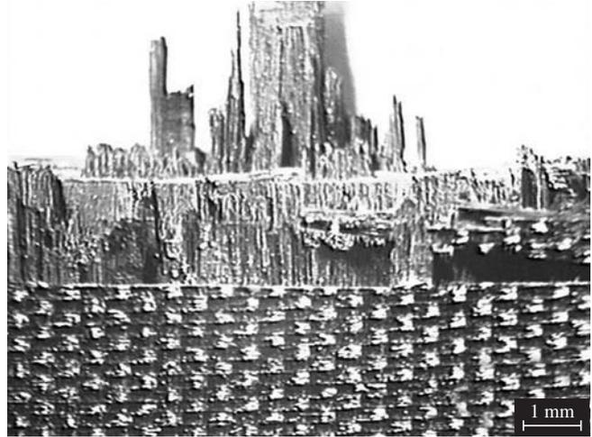
Figure 11. F584/8HS specimen after tensile test, (10x).
