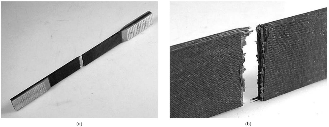
**Figure 7.** F584/8HS laminate: a) specimen tested; and b) detail of the failure mode type LGM (**Lateral Gage Middle**).
