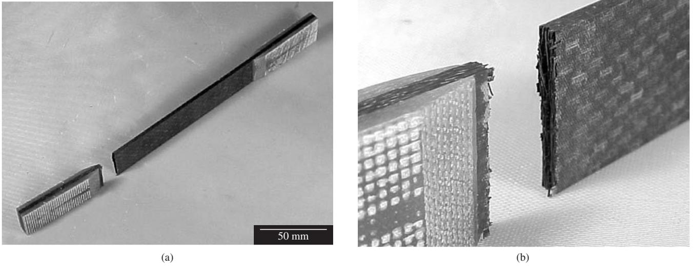
**Figure 5.** F155/8HS laminate: a) specimen tested; and b) detail of the failure mode type LAB (**Lateral At grip/tab Bottom**).
