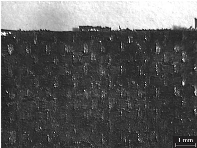
Figure 9. F584/PW specimen after tensile test, (10x).
