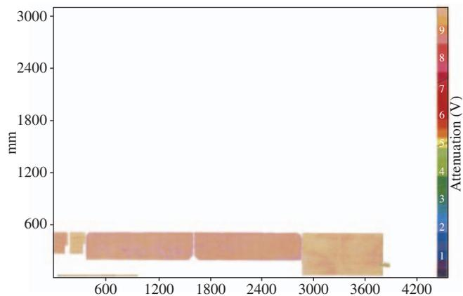
Figure 3. Typical C-Scan ultrasonic images after laminates molding.
