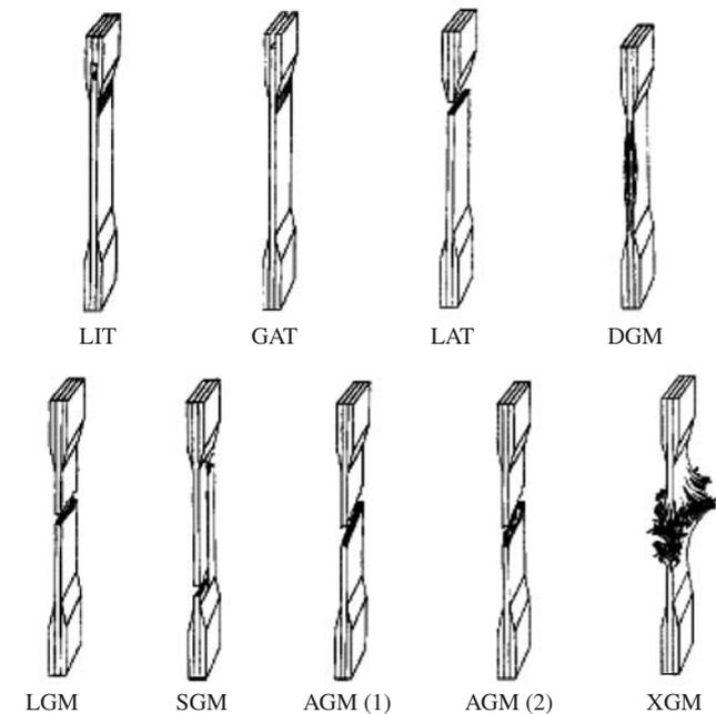
Figure 2. Representation of some typical failure modes in tensile tests of composites<sup>20</sup>.
