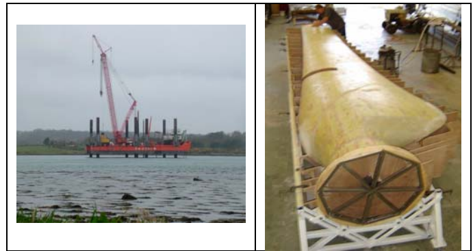
Figure 14. MCT SeaGen geo technical testing at Strangford for foundation design and a blade mold
