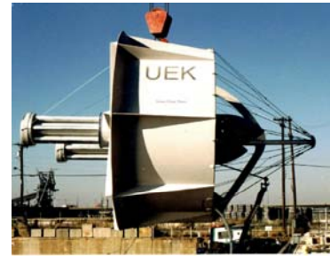
Figure 110. UEK Shrouded Turbine
