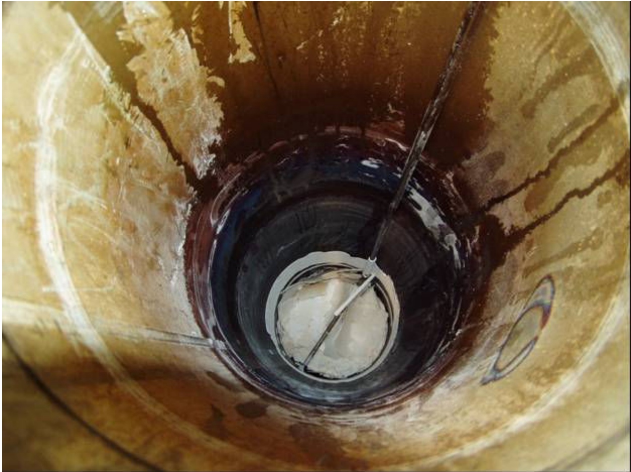
Figure 20 - Calcium Carbonate Crust in Cold Tank After Breakup
