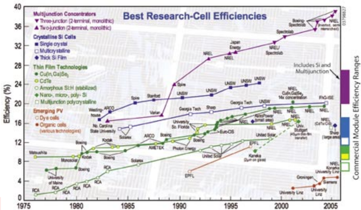
Fig. 3.1.2-1 Historical laboratory cell efficiencies, compared with 2005 module efficiencies.
