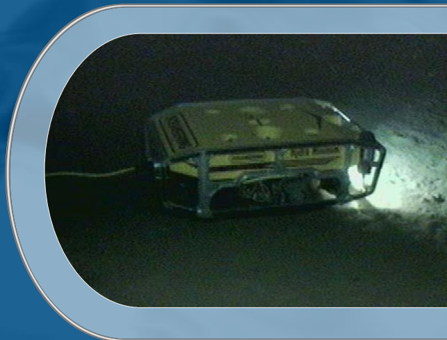
The Minimum ROV supporting drilling operations at 9,347 fsw.
