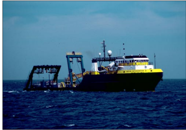
Ocean Intervention II plug and abandonment deck layout, with 60 T subsea intervention A-frame
