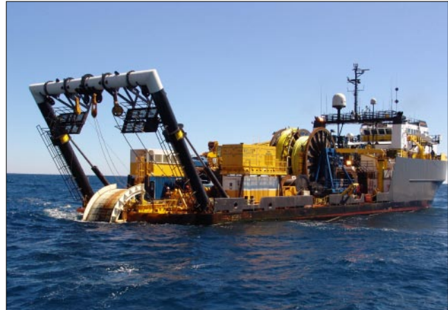
Flexible flowline and umbilical installation spread Photo by RCMG, LLC
