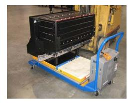
Figure 1 – Tesla Roadster battery pack
