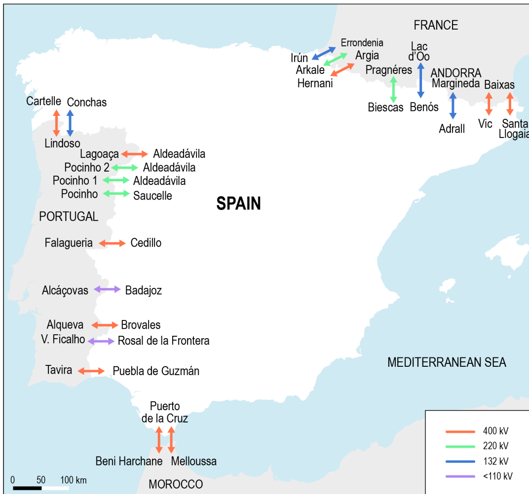
Figure 7.4 Spain's current interconnections with neighbouring countries
