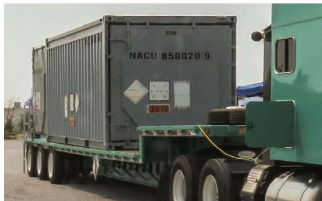
Truck carries transport package for research reactor fuel.
