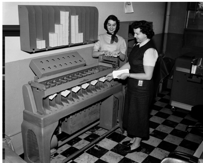
Historical photo: The card reader sorted keypunched cards for data entry to the first mainframe computer at Fernald, an IBM1620, located in the Accounting Division. Photo posted at https://www.flickr.com/photos/departmentofenergy/29242374641/in/photostream/ .
