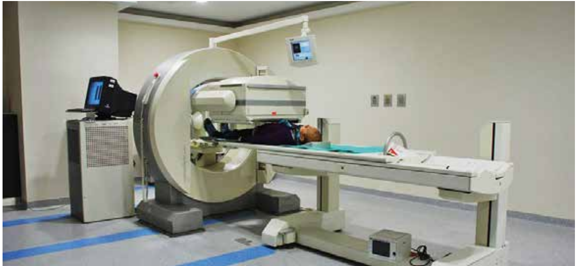
A gamma camera traces and detects radiopharmaceuticals inside of a patient in order to produce diagnostic images.
