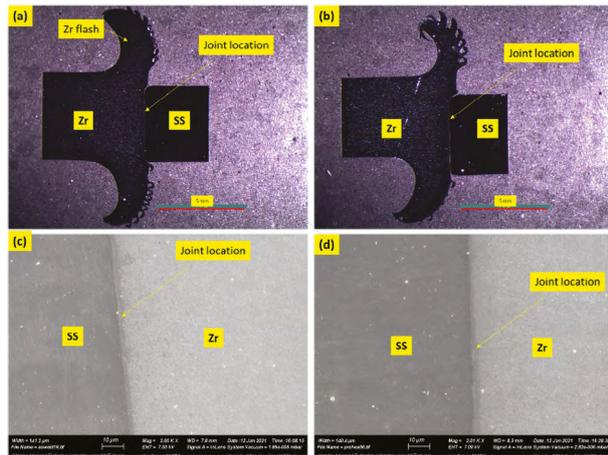
Note: Both samples were produced at 1200 rpm, using a burn off pressure of 59.5 MPa and a burn-off length of 1.0 mm, but sample 7 was preheated to 600°C for 30 minutes before welding.
