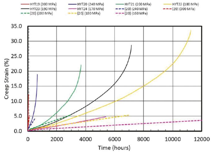
Note: The solid lines show creep strain deformation of PM/HIP 316L austenitic stainless steel at 600°C in air compared to the conventionally forged material. Source: Data from Jacobs (United Kingdom). New results (not yet published) presented at the VHTR MAT PMB meeting in September 2022.
