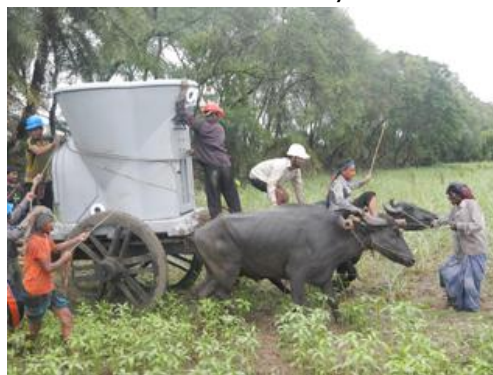
Transporting Sonic Detection and Ranging (SODAR) device for remote wind measurement in Bangladesh. Photo by Harness Energy
