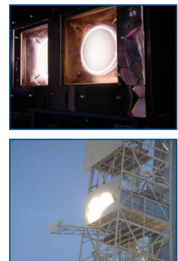
Below: Dual-chamber HYDROSOL-I (Conti) (top) and HYDROSOL-II reactors (bottom) operating under concentrated solar irradiation
