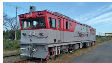
SMART-i is a dedicated maintenance railcar equipped with Shinkansen track equipment monitoring systems.
