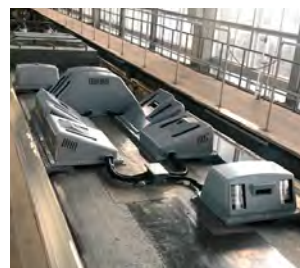
East-i is an electricity and track general inspection railcar equipped with overhead wire equipment monitoring systems.
