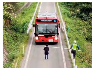
Automated stopping test assuming the entry of people into a dedicated BRT road
