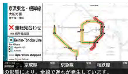
Detail of LCD guidance display for emergency situation
