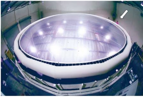
Figure 6: Inflatible Antenna Experiment reflector during ground tests. For scale, note the person on the right wearing a red shirt.
