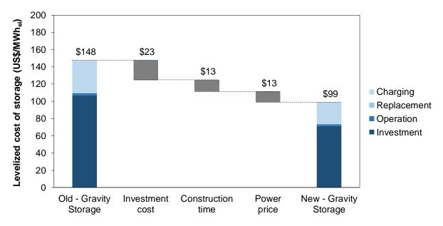
Figure 5 – LCOS reduction due to new construction technology, alternative design and updated power cost assumption for a 8 GWh / 1,000 MW Gravity Storage system compared to report from November 2017 [6].
