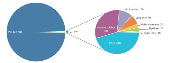
Figure 2 – Global installed electricity storage capacity in 2010 in MW [1]; PSH – Pumped Hydro Storage, CAES - Compressed Air Energy Storage
