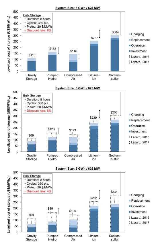
Figure 7 – Impact of different discount rate assumption (8%, 6%, 4%) on LCOS for 5 GWh / 625 MW systems. Discount rates reflect energy and infrastructure projects in recent years (8%), low current interest rates (6%) and the potential satisfaction with returns in low risk and regular, stable revenue investments (4%). Values compared to results from studies by Lazard [3,4]. Dashed rectangles reflect respective LCOS at 8% discount rate and are included as visual guidance.
