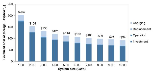
Figure 4 – Levelized cost of storage for Heindl Energy Gravity Storage systems for different system sizes. Energy storage capacity ranges from 1 to 10 GWh. Discharge duration is kept constant at 8 hours, so respective power capacity ranges from 125 to 1,250 MW. Different shading of blue indicates LCOS components, namely power, replacement, operation and investment cost.
