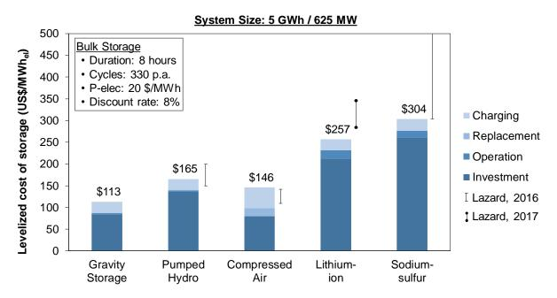
Figure 1 – LCOS in US\$/MWhel for investigated bulk storage technologies of 5 GWh system size, 8 hours discharge duration, 330 full equivalent charge cycles per year, electricity price of 20 US\$/MWh and 8% discount rate. Values are compared to results from studies by Lazard. Only lithium-ion among technologies considered in 2017 study.
