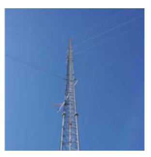
Meteorological masts or towers are typically 60 or 80 meters tall and have monitoring equipment at multiple heights. These towers use anemometers, wind vanes, and temperature sensors to measure the wind speed, wind direction, and temperature. This wind resource data is collected and stored by a data logger for later analysis.
