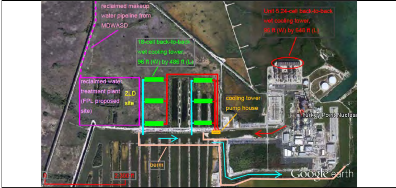
Figure 12. 54-Cell Back-to-Back Mechanical Draft Cooling Towers
