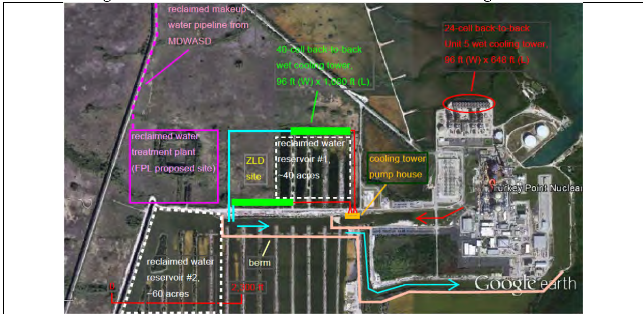
Figure 13. 40-Cell Back-to-Back Mechanical Draft Cooling Towers 84
