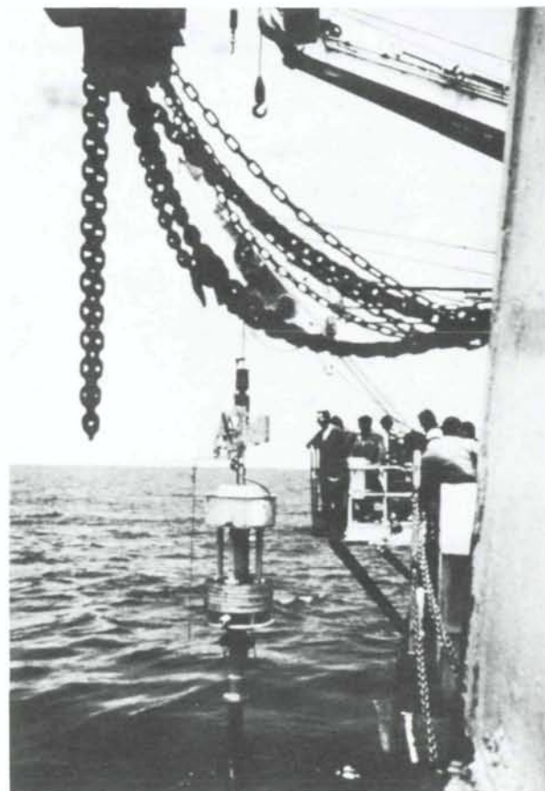
National and international programmes have improved knowledge about the potential impact of deep sea disposal of radioactive waste. Shown here, about to be submerged, is a new type of "sediment corer" to sample the 30 upper metres of seabed sediment. (Credit: CEA/DPT)
