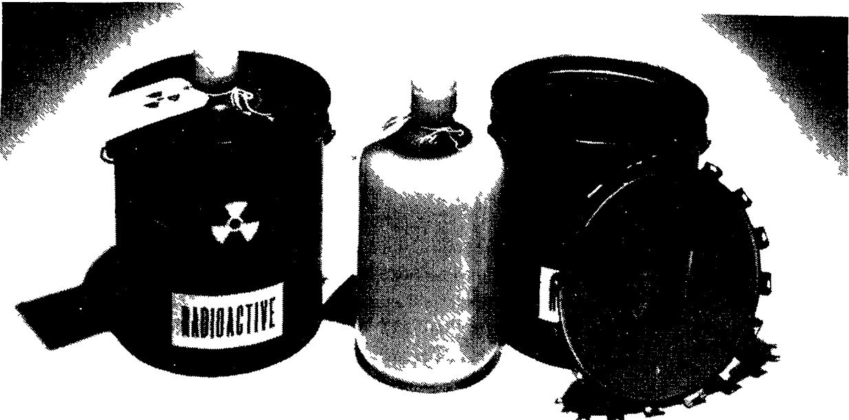
FIG 2 Liquid waste collection containers
