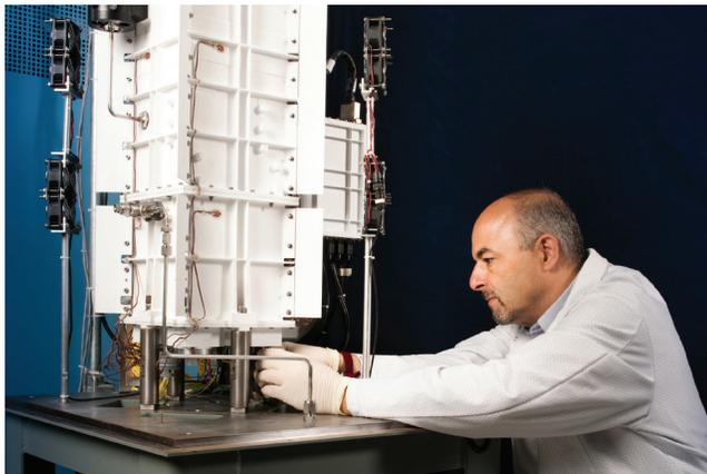
An engineer works on an engineering test unit of the ASRG. Such test units (with non-nuclear heat sources) have operated for a total of more than 33,000 hours in the laboratory over more than a decade of increasingly integrated development work.
