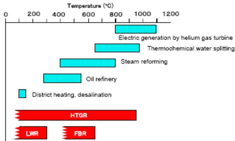
FIG. C-1. Range of operating temperatures and process heat requirements
