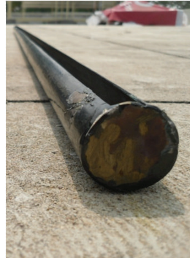
FIGURE 13: Pictorial view of absorber design in CPC-TSS.
