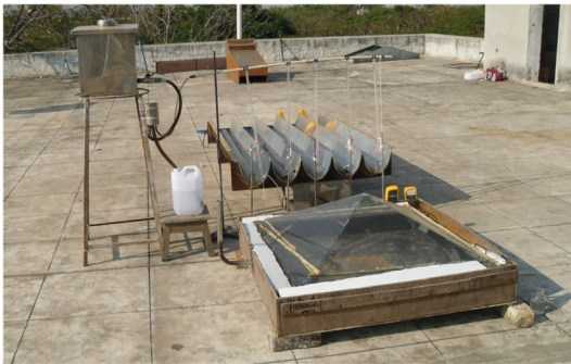
FIGURE 16: Pictorial view of CPC-pyramid solar still design.
