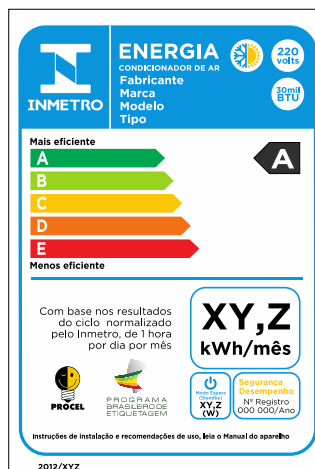
Figure 1. Energy Conservation National Label and PROCEL Label used for air conditioners in Brazil (PROCEL and INMETRO)
