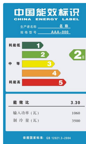
Figure 1. Energy Information Label (mandatory) and Energy Conservation Label (voluntary) adopted in China for AC appliances (Zhou, 2008)
