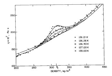
Fig. 9 Viscosity data for nitrogen in the critical region as measured by Zozulya and Blagoi (1974). The curves indicate the values calculated from the proposed viscosity equation with  $T_c = 126.201$  K.
