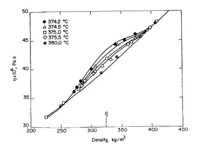
Fig. 11 Viscosity data for steam in the critical region (Rivkin et al. 1975; Watson et al., 1980). The curves indicate the values calculated from the proposed viscosity equation with  $T_{\rm c}=647.033$  K.
