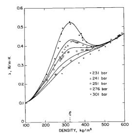
Fig. 8 Thermal conductivity data for steam in the critical region at four different isobars, measured by Sirota et al. (1974, 1976). The curves indicate the values calculated from the representative equation proposed in this report.
