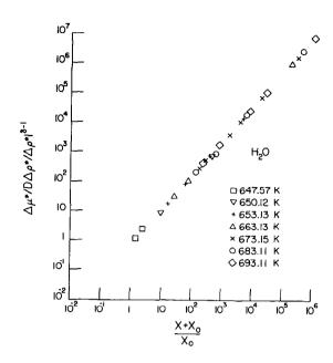
Fig. 3 Scaled chemical potential data for steam as a function of  $y = (x + x_0)/x_0$ . Reduction parameters are taken from Table IV.
