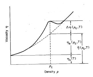
Fig. 6 Schematic representation of the viscosity  $\eta(\rho,T)$  as a function of the density  $\rho$  at a temperature slightly above the critical temperature.
