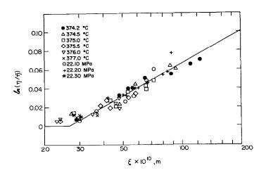
Fig. 12 Log-log plot of the viscosity ratio  $\eta/\bar{\eta}$  as a function of the correlation length  $\xi$  for steam in the critical region.
