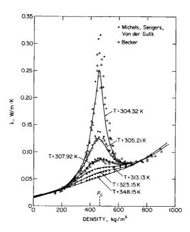
Fig. 7 Thermal conductivity data for carbon dioxide in the critical region along isotherms as a function of density. The curves indicate the values calculated from the representative equation proposed in this report.
