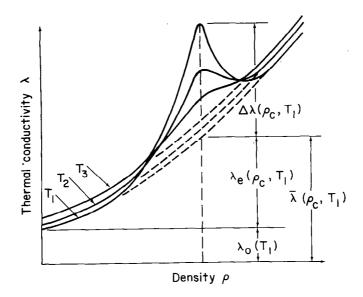
Fig. 5 Schematic representation of the thermal conductivity  $\lambda(\rho,T)$  as a function of the density  $\rho$  at three supercritical temperatures  $T_1 < T_2 < T_3.$
