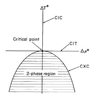
Fig. 1 Special paths in the  $\Delta T^*$  versus  $\Delta \rho^*$  plane for the definition of critical power laws.
