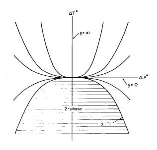
Fig. 2 Curves of constant y in the  $\Delta T\star$  versus  $\Delta\rho\star$  plane.
