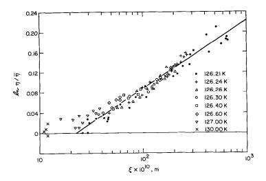
Fig. 10 Log-log plot of the viscosity ratio  $\eta/\bar{\eta}$  as a function of the correlation length  $\xi$  for nitrogen in the critical region.
