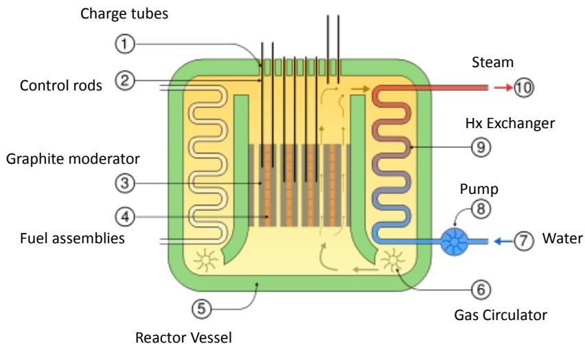
In some advanced and developing HTGR designs, the hot helium is piped directly to a gas turbine to generate electricity. Because of the higher coolant temperatures, HTGRs operate at a higher thermal efficiency than water cooled reactors and are able to use the same steam turbines as conventional fossil power plants. Two attempts at nuclear superheating steam were made during the AEC's power demonstration program, but proved unsuccessful.
