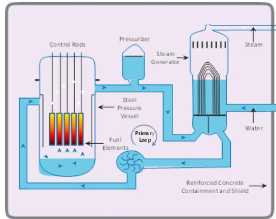
Pressurized Water Reactors operate with a “primary loop” and a “secondary loop”. Water in the primary loop circulates through the reactor core where it is heated. The primary coolant then flows through a steam generator and transfers its heat to water on the opposite side of tubes (secondary loop),
