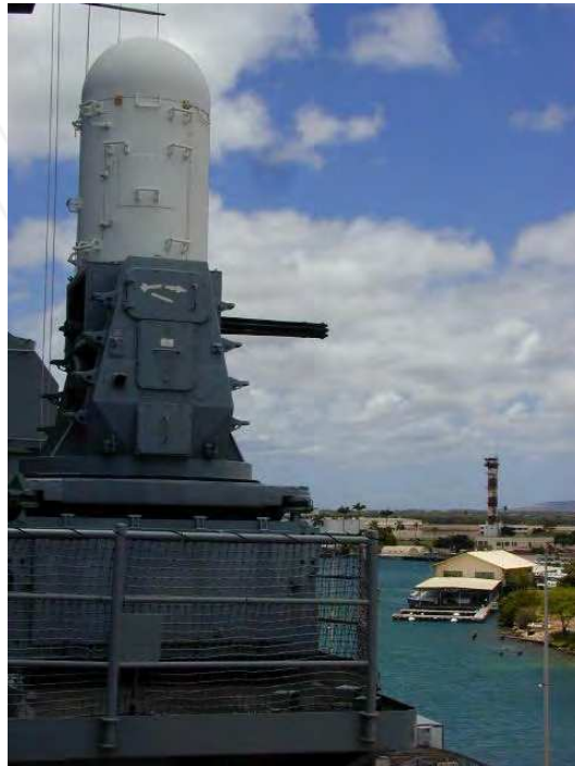
Fig. 10. The Phalanx radar-guided gun, nicknamed as R2-D2 from the Star-Wars movies, is used for close-in ship defense. The radar controlled Gatling gun turret shooting tungsten armor-piercing, explosive, or possibly depleted uranium munitions on the USS Missouri, Pearl Harbor, Hawaii. (Photo: M. Ragheb).
