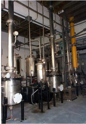
Figure 5: Uranyl nitrate purification pilot plant.
