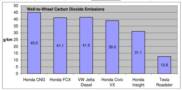
Again, the electric car shines – from the perspective of CO<sub>2</sub> emissions, it is three times better than the hybrid car, and nearly four times better than the hydrogen fuel-cell car.
