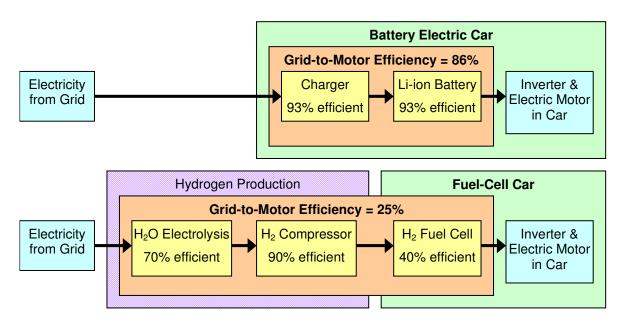
It is obvious that when we start with electricity (however it is produced), it is hard to beat the 86% efficiency of the currently available lithium-ion batteries and chargers. Even when we assume extremely high efficiencies for electrolysis, compression, and the fuel cell, the fuel-cell car requires more than three times as much electricity from the grid to drive the same distance.
