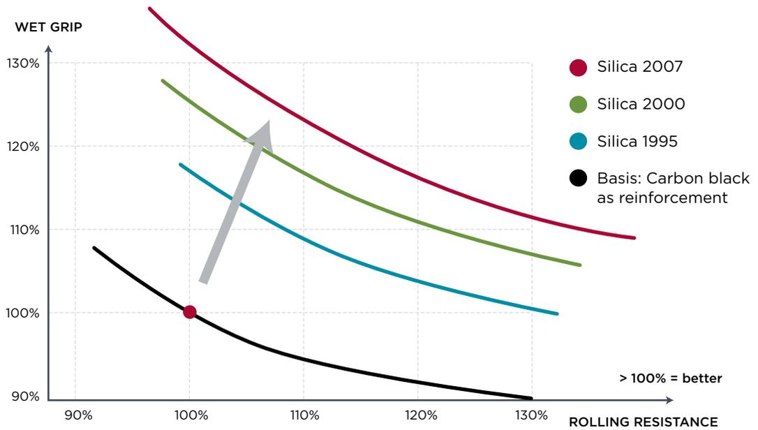
**Figure 3.** Wet grip versus rolling resistance.
