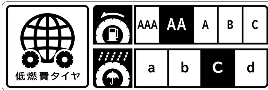
**Figure 7.** Sample Japanese tire label. Left, low-energy tire logo; upper right, RRC grade; lower right, wet-grip grade.
