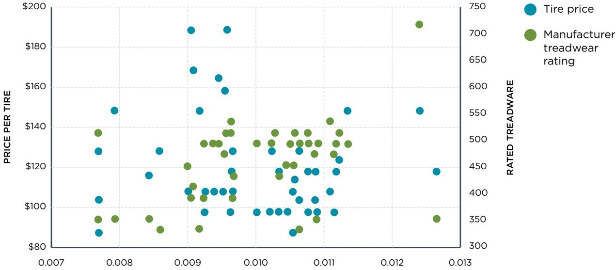
**Figure 4.** Tire rolling resistance versus price and relative rated treadwear for (A) size 195 tires and (B) size 265 tires. Data from California Energy Commission (2010).
