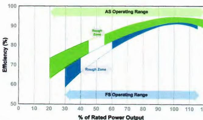
Figure 2. Comparison of Efficiency Curves in Generation Mode for FS (Blue) and AS (Green) PSH Units (adapted from USACE 2009<sup>6</sup>).
