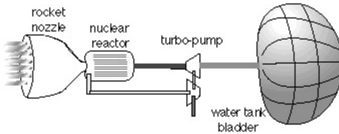
Figure 5. Nuclear Thermal Rocket (NTR) uses nuclear reactor to heat propellant (water or liquid hydrogen, LH<sub>2</sub>). Rocket nozzle is bolted directly on to reactor. Bleed gas turbo pump forces propellant into reactor. LH<sub>2</sub> NTR's would deliver 800 - 900 seconds specific impulse and run at power densities ~ 300 megawatts per ton of rocket.
