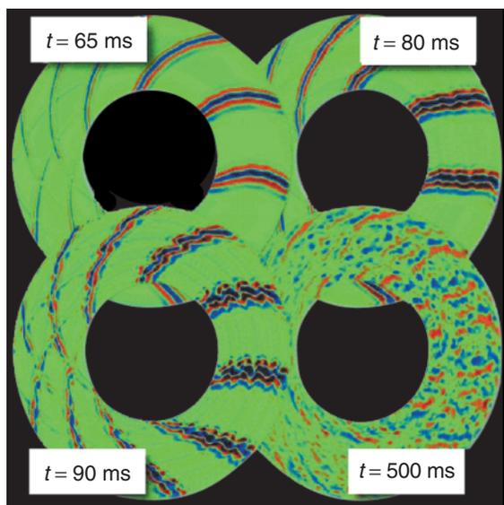
This simulation, done by Livermore collaborator General Atomics of San Diego, California, with the GYRO code, shows a cross section of a tokamak over time ( $t$ ) in microseconds (ms). The color contours indicate microturbulent fluctuations in the plasma density. The center sections have been removed to facilitate comparison.
