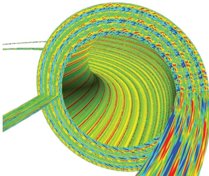
Part of the cross section of a tokamak plasma. The color contours indicate microturbulent fluctuations in the plasma density. Livermore’s PG3EQ code, which was used to produce this simulation, models a “tube” of magnetic flux as it wraps once around the tokamak poloidally, or the short way around. Toroidal symmetry was then used to displace this flux tube and fill the annulus.
