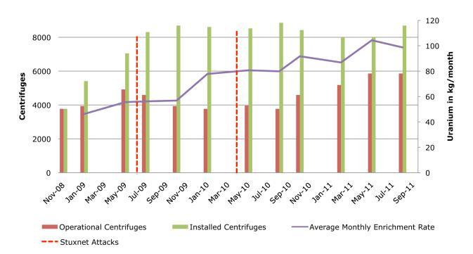
Figure 2. Enrichment Rate vs. Operational Centrifuges at Natanz FEP
