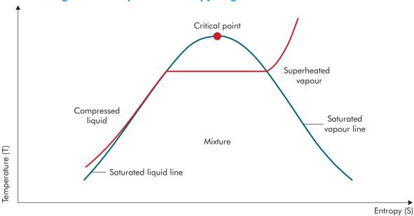
Figure I.3: Temperature-entropy diagram for steam and water
