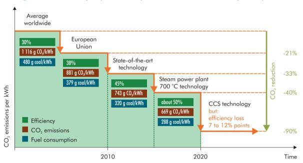
Figure 4.5: Efficiency improvement potential at hard coal-fired power plants
