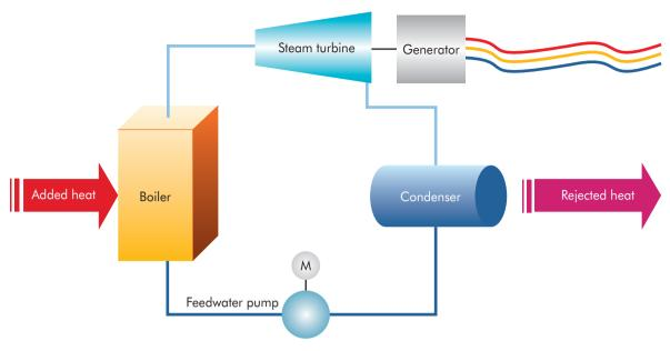
Figure I.2: Basic representation of the vapour-power cycle
