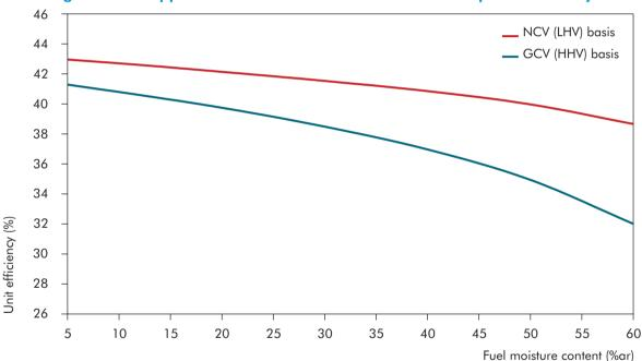
Figure 3.10: Approximate influence of coal moisture on plant efficiency
