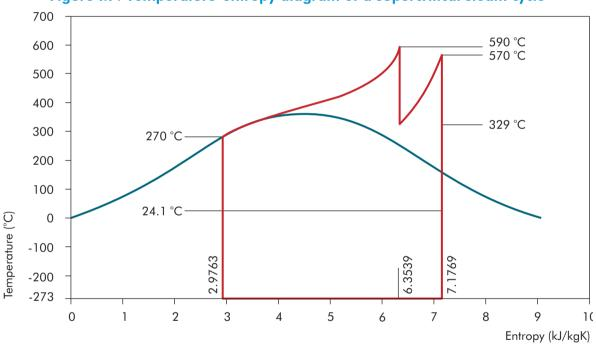
Figure 1.7: Temperature-entropy diagram of a supercritical steam cycle
