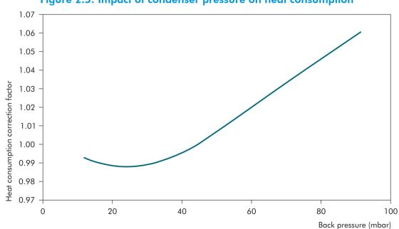
Figure 2.5: Impact of condenser pressure on heat consumption
