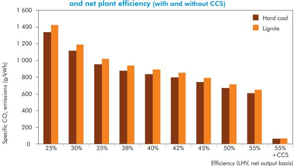
Figure 2.8: Example of relationship between CO<sub>2</sub> emissions and net plant efficiency (with and without CCS)
