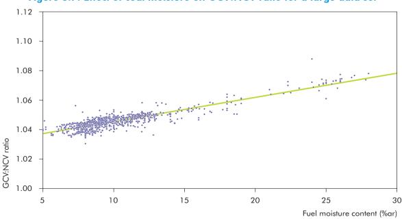
Figure 3.7: Effect of coal moisture on GCV:NCV ratio for a large data set
