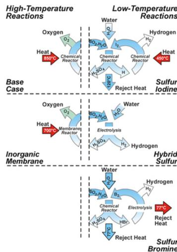
Figure 2.6-1. Sulfur-Based Thermochemical Cycles (Ref. 14)
