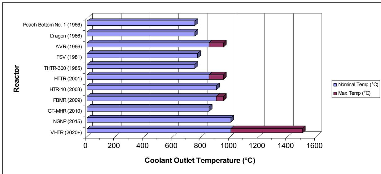
Figure 4.2-1. HTGR Coolant Outlet Temperatures
