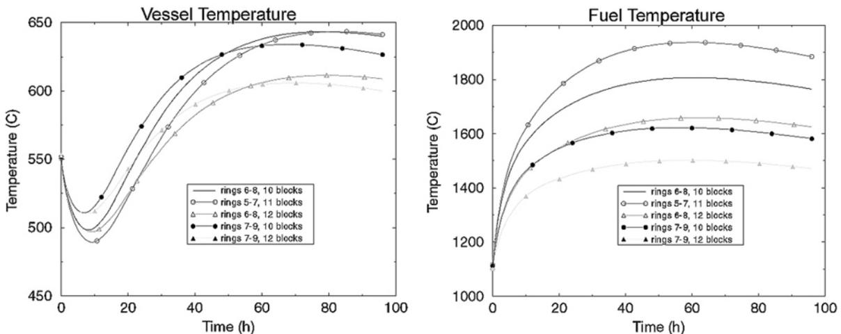
**Figure 2.8-1. VHTR Peak Temperatures During Accident (Ref. 23)**
