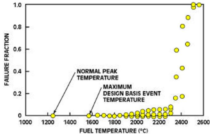
**Figure 3.1-1. SiC Coated Fuel Particle Temperature Capability (Ref. 19)**
