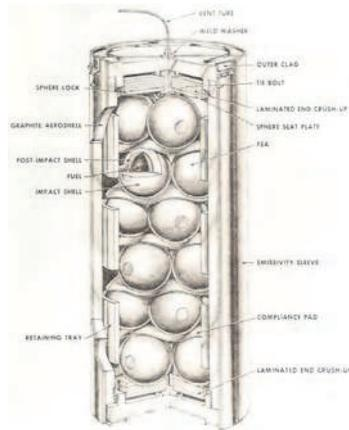
Fig. 20. MWH-RTG heat source.
