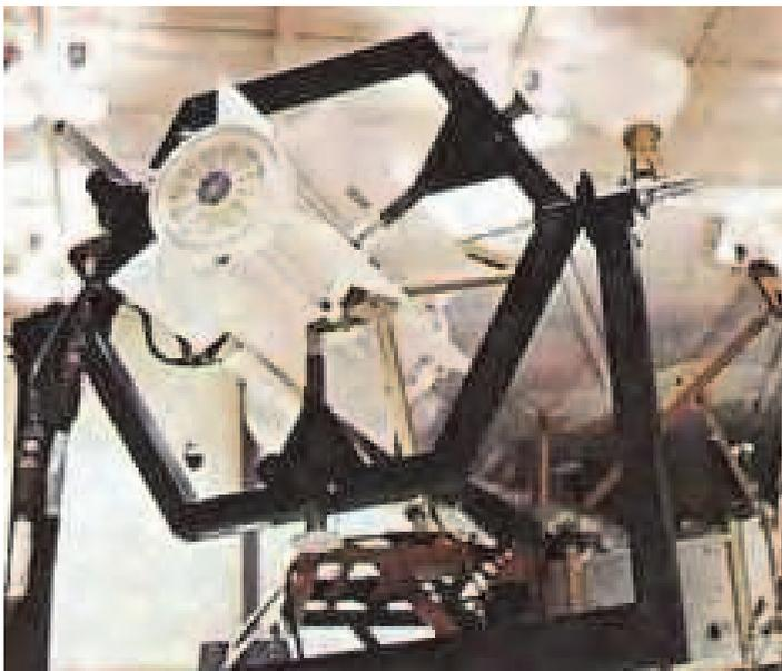
Fig. 12. SNAP-19s installed on Pioneer.
