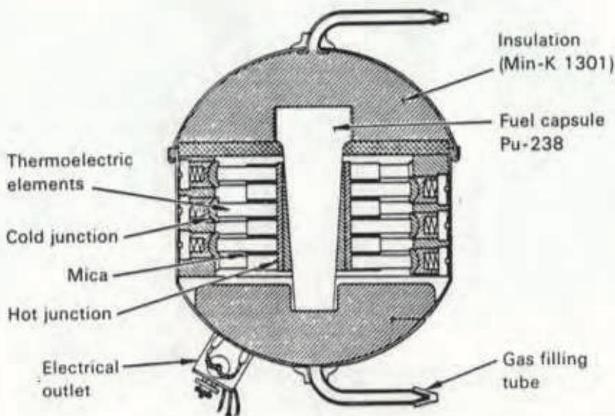
Fig. 6. SNAP-3B Schematic.
