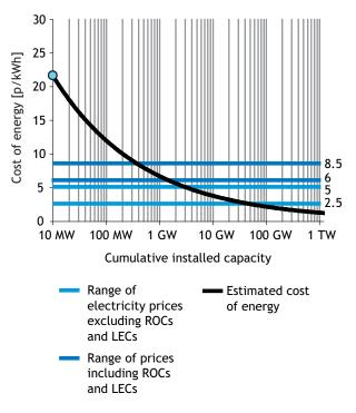
Note: Curves implicitly includes a gradually falling discount rate from 15% to 8%. Source: Entec
