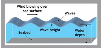
Wave energy occurs in the movements of water near the surface of the sea. Waves are formed by winds blowing over the sea surface, and the water acts as a carrier for the energy. The amount of energy in waves depends on their height and period (the time between successive peaks). The annual average power per unit length of wave crest (e.g. 40 kW/m) is a first indicator of how energetic a particular site is.
