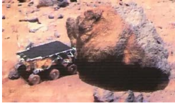
Figure 16. Mars Sojourner sampling a Martian rock. It uses Radiosotopes Heating Units (RHUs) to maintain a desirable operating temperature of its electrical components during the cold Martian nights.
