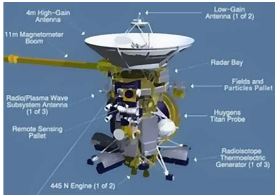
Figure 11. The Cassini Space craft showing its three thermoelectric radioisotope generators.
