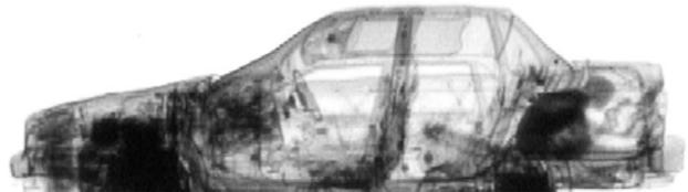
Figure 22. Car image using the VACIS<sup>TM</sup> vehicle inspection system [SAIC, 2004].
