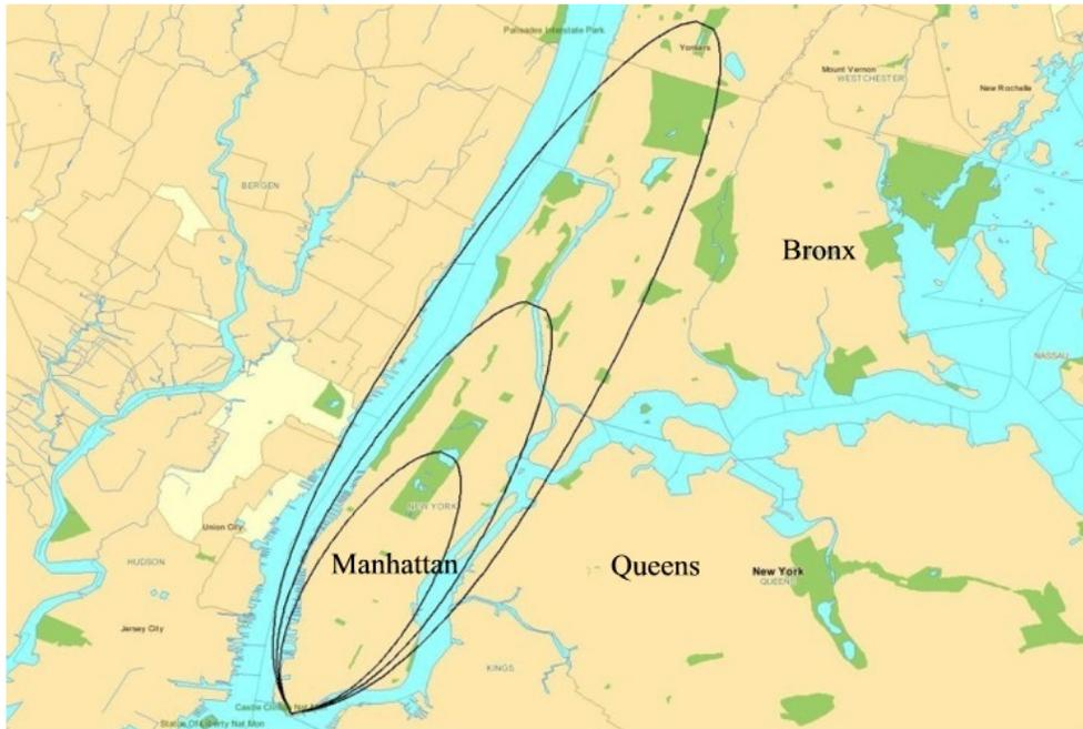
Figure 7. Simulation of a dirty bomb using an industrial cobalt source normally used for food irradiation. The inner contour shows contamination at radiation levels equal to the permanent exclusion zone at Chernobyl. The middle contour equals the permanently controlled zone and the outer contour the periodically controlled zone. [FAS, 2002].
