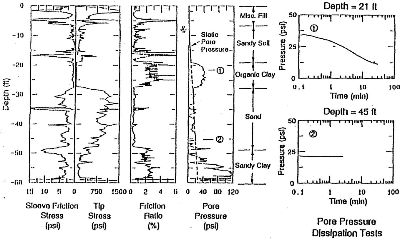
Figure 1: Typical Soil Cone Penetrometer Data
