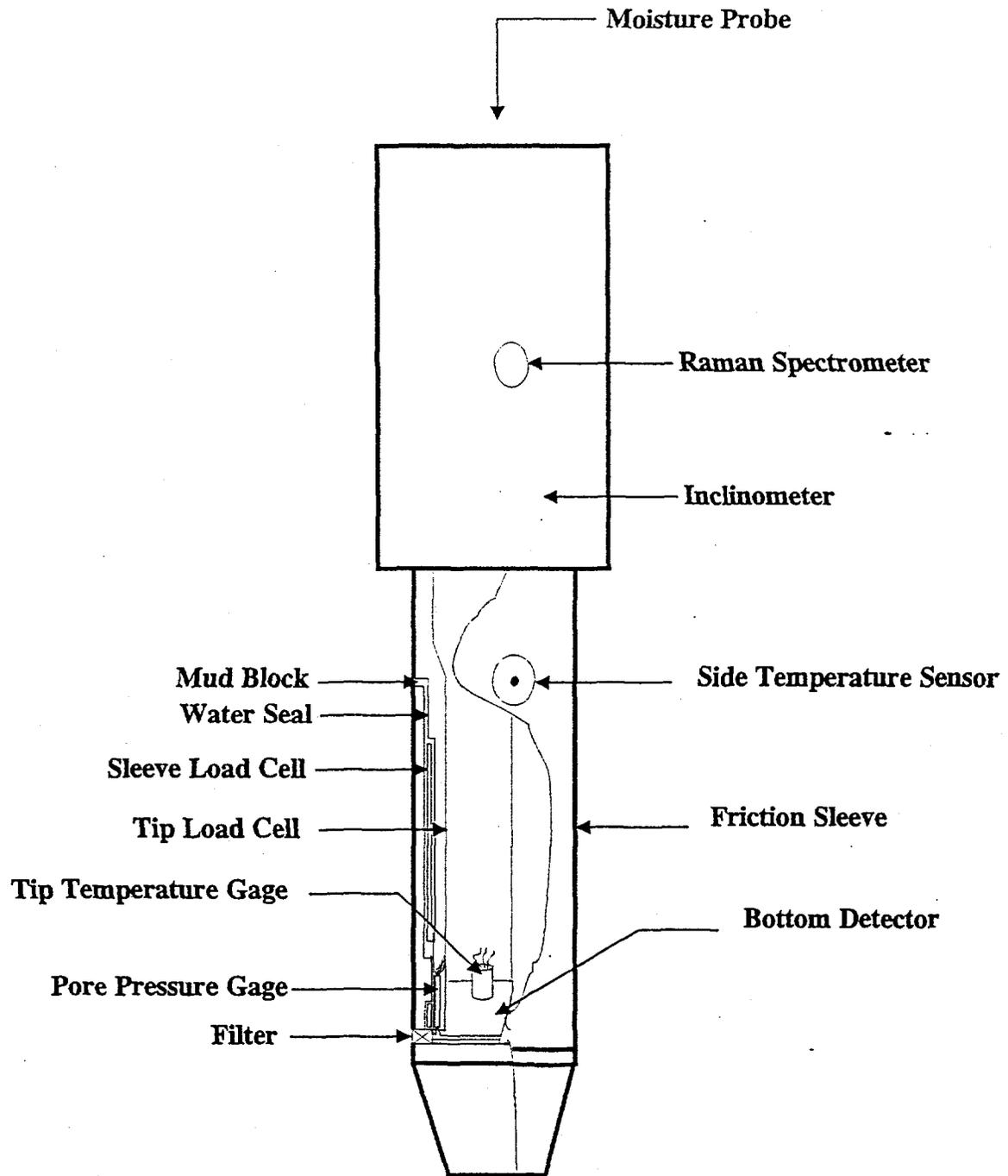
**Figure 2: Cone Penetrometer Sensor Tip Schematic**
