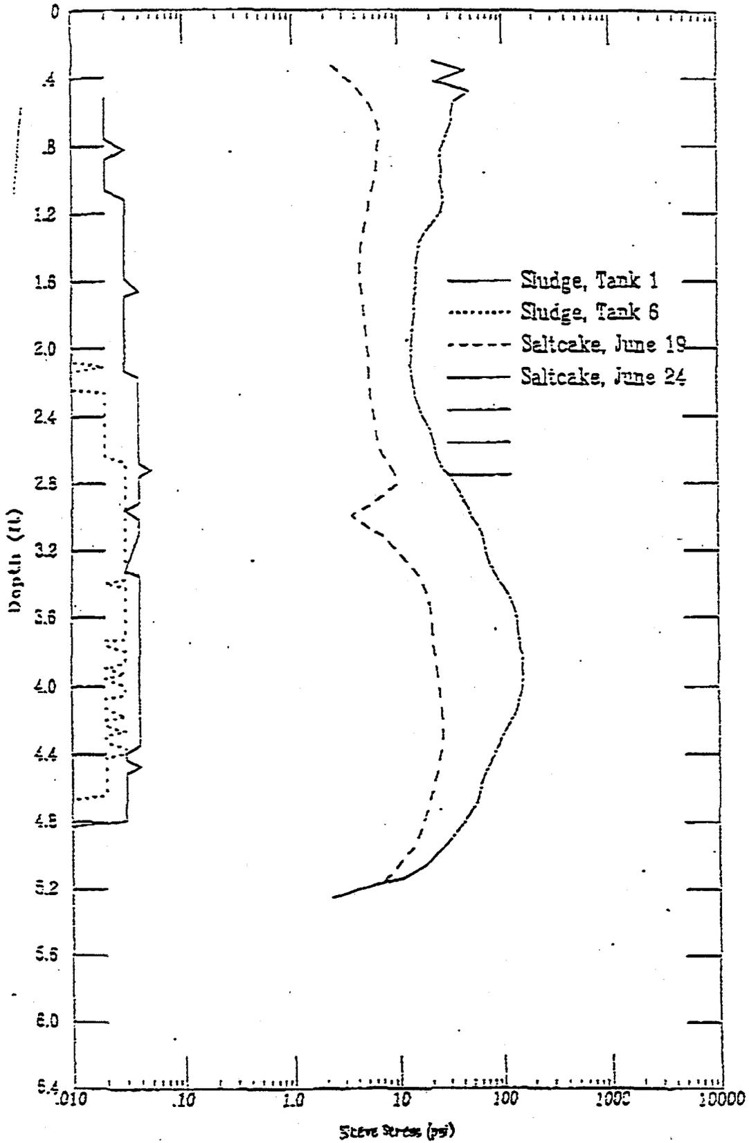
SIMULANT CHARACTERIZATION - SLUDGES
